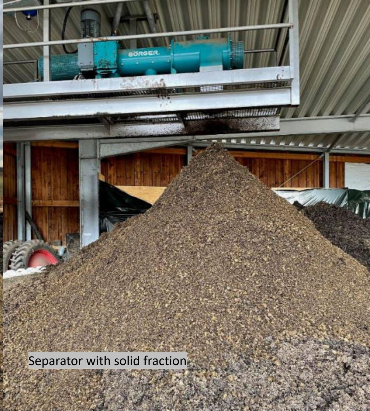
Separator with solid fraction
