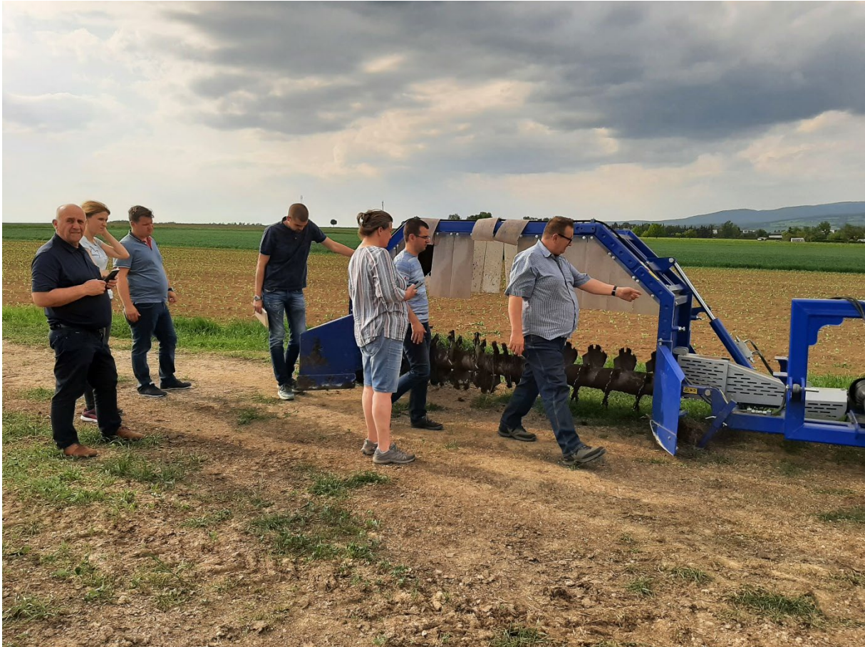
Picture 2: Compost turning machine, Werner Vogt-Kaute
